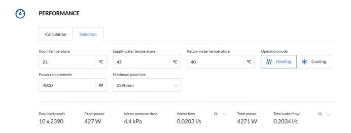
In the selection section, the idea is to calculate the total number of panels required when the power is known. The set values here are room temperature: 21 degrees, supply water temperature: 45 degrees, and return water temperature: 40 degrees. The power requirement is 4000 W and the maximum panel size on the site in question can be ItuGraf panels of 2390 mm in length.
