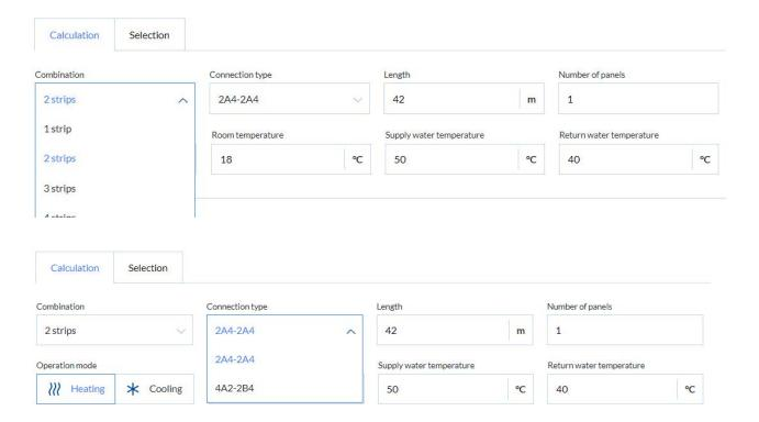
In the calculation section, you select the number of ItuString+ radiant ceiling panels (320 mm wide), which can be between 1 and 4 panels in parallel, and the connection type.
