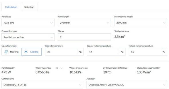
Two ItuGraf 595 mm x 2990 mm panels have been selected for cooling. The panels are connected in parallel. The set values are room temperature: 25 degrees, supply water temperature: 14 degrees, and return water temperature: 16 degrees. The calculation gives the capacity, flow and pressure loss for a pair of panels connected in parallel, as well as the temperature difference and output per square metre.
