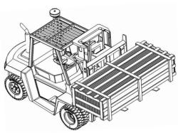
2. Radiant panels can be unloaded from a lorry using a forklift truck. To avoid damage, transport boxes must be moved one at a time. When lifting a box, place the forks of the forklift truck in the middle of the box. The forks must be longer than the depth of the box. Make sure that the transport box is balanced!
