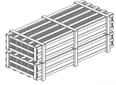
Itula radiant panels are delivered in wooden transport boxes. Boxes should always be lifted to be unloaded, never pushed or pulled. No other load must be placed on top of the boxes when they are being lifted.
