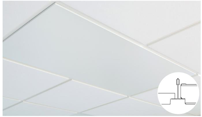
ItuGraf® Model E has been designed to match the E24 edge. The E edge has a recessed visible grid, creating a ceiling with a shadow effect. The visible surface of each tile is 10 mm below the grid.
