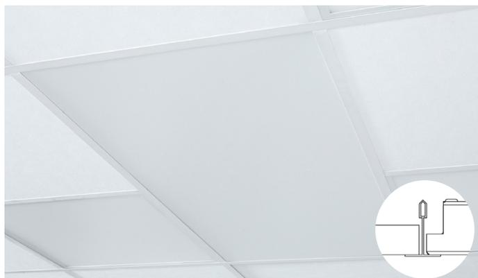
ItuGraf® Model A integrates with the A edge in the Focus and Master ceiling systems. The A edge has a visible grid and easily demountable tiles. Unlike with the other edges, the ItuGraf® Model A ceiling can be used with the T24 grid and also with the T15 grid.
