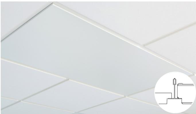
ItuGraf® Model E has been designed to match the E edge in the Focus and Master ranges. The E edge has a recessed visible grid, creating a ceiling with a shadow effect. The visible surface of each tile is 10 mm below the grid. All of the tiles are easily demountable.
