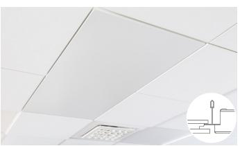
ItuGraf® Model M has been designed to match the M edge. The M edge design has concealed support edges to create a distinctive floating appearance. The suspension grid is approximately 14 mm above the visible surface of the tile, which gives the impression that each tile is individually suspended. All of the tiles are easily demountable.
