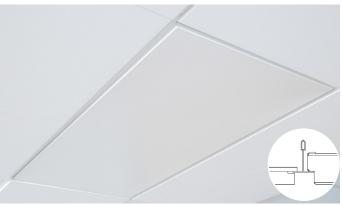
ItuGraf® Model Lp fits together with the Lp edge in the Focus range. The Lp edge semi-concealed grid system can be used for highlighting direction in a room. The longer sides have a wide gap between the tiles while the tile connections on the shorter sides are concealed.
