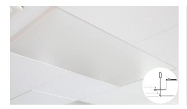
ItuGraf® Model Ds can be used with the Ds edge in the Focus and Master ranges. The Ds edge is suitable for applications where a suspended ceiling with a concealed grid is required. The tiles have a symmetrical edge design. The ceiling has an even appearance, with the bevelled edges forming a discreet groove between the tiles. The tiles are easily demountable.
