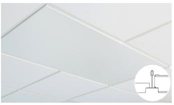
ItuGraf® Model E has been designed to match the E24 edge. The E edge has a recessed visible grid, creating a ceiling with a shadow effect. The visible surface of each tile is 10 mm below the grid.
