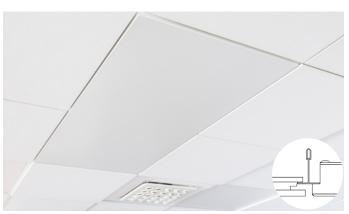
ItuGraf® Model Dg has been designed to match the Dg edge in the Focus range. The Dg edge design has concealed support edges to create a distinctive floating appearance. The suspension grid is approximately 14 mm above the visible surface of the tile, which gives the impression that each tile is individually suspended. All of the tiles are easily demountable.
