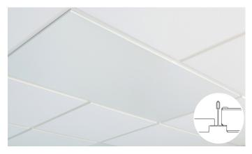
ItuGraf® Model E has been designed to match the E edge in the Focus and Master ranges. The E edge has a recessed visible grid, creating a ceiling with a shadow effect. The visible surface of each tile is 10 mm below the grid. All of the tiles are easily demountable.
