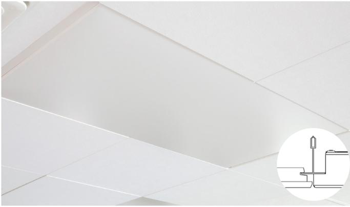
ItuGraf® Model X can be used with the X edge. The X edge is suitable for applications where a suspended ceiling with a concealed grid is required. The tiles have a symmetrical edge design. The ceiling has an even appearance, with the bevelled edges forming a discreet groove between the tiles. The tiles are easily demountable.
