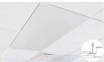
ItuGraf® Model M has been designed to match the M edge. The M edge design has concealed support edges to create a distinctive floating appearance. The suspension grid is approximately 14 mm above the visible surface of the tile, which gives the impression that each tile is individually suspended. All the tiles are easily demountable.
